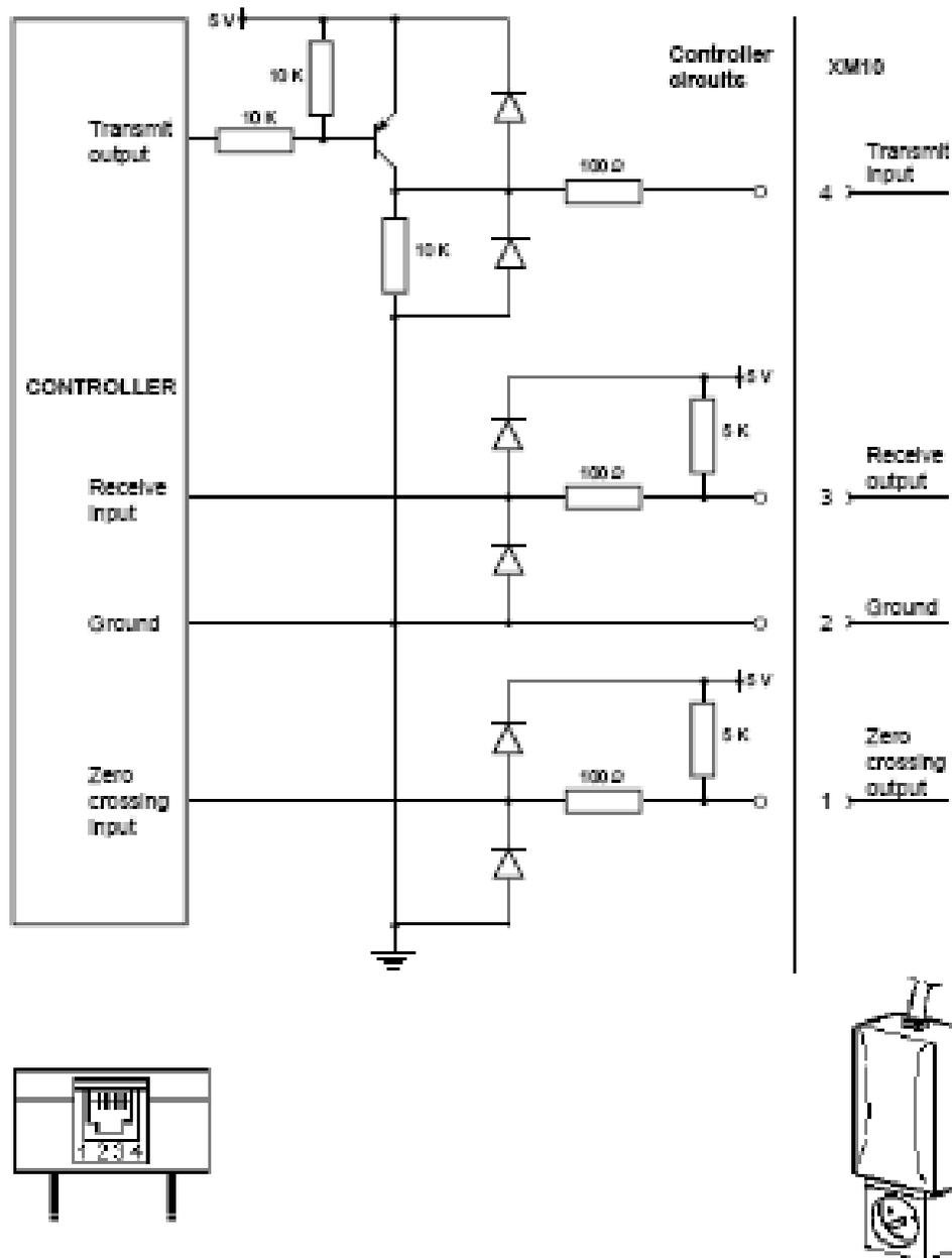
Connection between the controller is via a standard modular phone jack, the connections for which are as follows:
