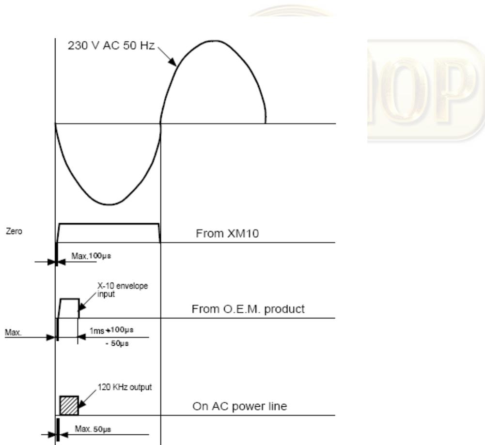
Figure 2: Transmit Timing Diagrams
